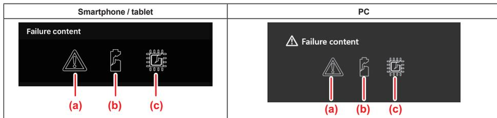
These icons indicate the type of battery's malfunctioning. The icon that corresponds to the malfunction is filled in. Regarding failures, ask the store where you purchased the product or Makita Service Center.
